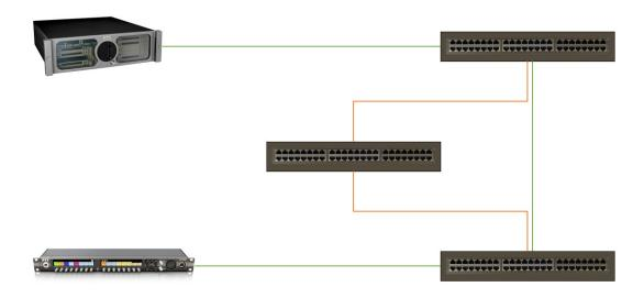
In this example, the direct connection between two switches has failed. As RSTP is active, the routes are known and another route is taken for communication between the devices. Also, there is only one back-up connection, but with RSTP there can be multiple routes available not just one or two.
