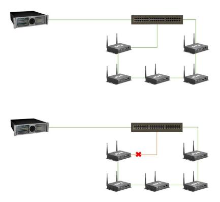
In this example, the devices are interconnected as a daisy chain loop. A daisy chain loop is easy and fast to install and can be used as an ad-hoc solution. In case of cable or device failure between devices, the communication path continues via the other end. If the device contains an Ethernet port(s) and fiber optic port(s) both marked as OMNEO, a combination of Ethernet and fiber can be used to extend the distance between the switch or router and first connected devices of the chain.
