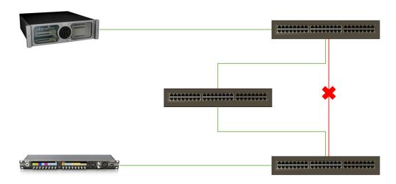
In this example, the ADAM M matrix has two connection by OMI interface to two different switches. The end-device, a keypanel single rack unit. uses OMNEO connected to two different switches. As well, the OMI as the keypanel can have only one Ethernet link active, with the second Ethernet link standby, the fastest route is used in order to reach the destination from the source. Between the switches, network information is shared about active links and end-devices. When one of the
