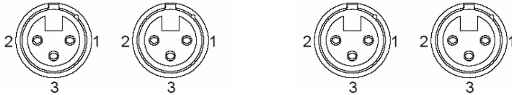
XLR 3p Female-panel Pinout
